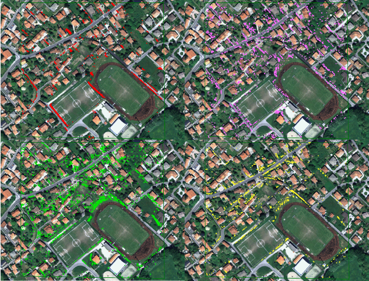
Sub test area 2, differences between DTM and raw Lidar data; legend like on the figure (0)
