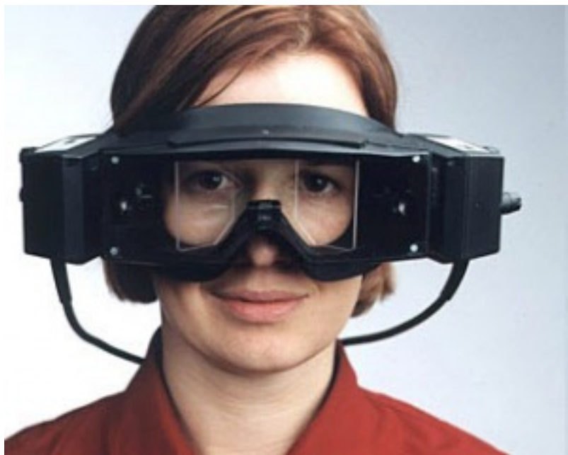
Rysunek 2.3: System 3D Video-Oculography®
