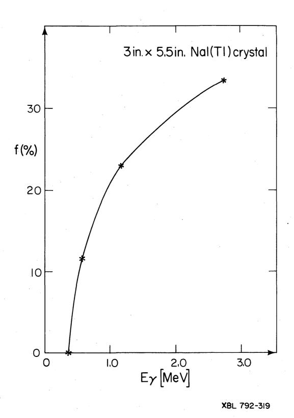
Fig. 6. Fraction of  $\gamma$  rays scattering into all neighboring crystals as a function of  $\gamma$ -ray energy for a 14 cm long, 7.6 cm diameter NaI crystal.
