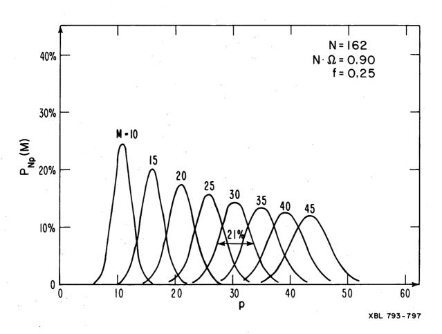
Fig. 3. Distribution of the number of hits, p, for a spherical shell of 162 counters with 90% efficiency and 25% Compton scattering.
