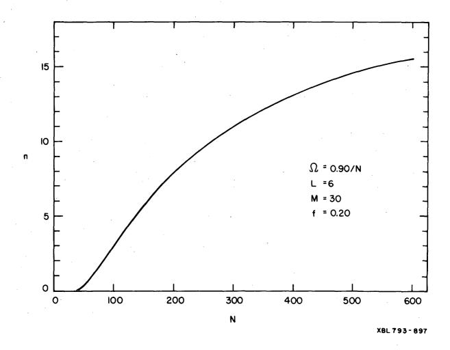
Fig. 4. The number of counters, n, without pile-up and no neighbor counters firing as a function of the total number of counters, N, with a total efficiency of 90%, a multiplicity of 30, f = 0.2, and six nearest neighbors for each crystal.
