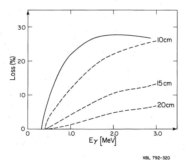
Fig. 5. Fraction of the  $\gamma$  rays which pass through a NaI shell of 10, 15, and 20 cm without any interaction (dashed lines). Fraction of  $\gamma$ -ray energy not detected, assuming one Compton scattering only, for 15 cm shell (full line).
