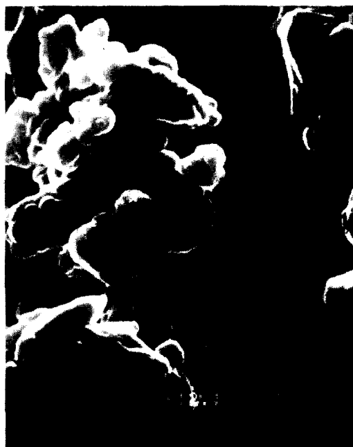
Fig. 2. SEM for AlN derived from [\text{HAlNH}]_n .
