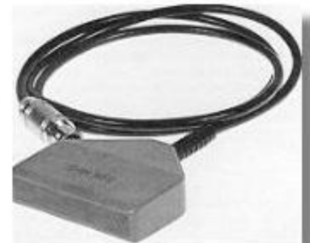
Bom's prototype 2.25 MHz linear array probe
