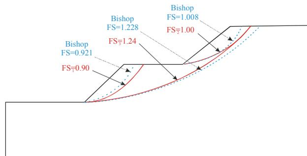
Fig.8. Several slip surfaces identified in benched slope by MSSR and LEM.
