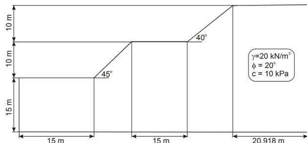
Figure 7. Benched slope problem geometry.
