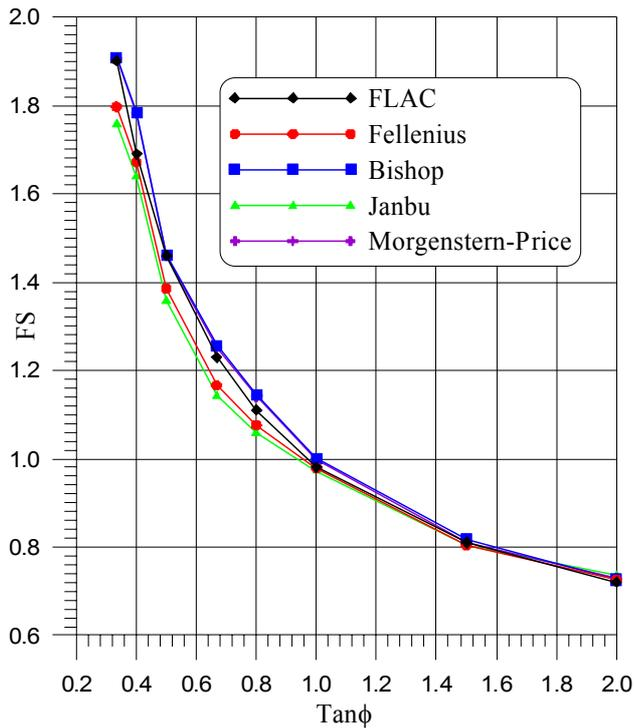
Figure 1. FS for embankment of height 25 m, friction angle  $\phi = 20^\circ$ , cohesion  $c = 30$  kPa for several sloping angles with SSR and LEM.
