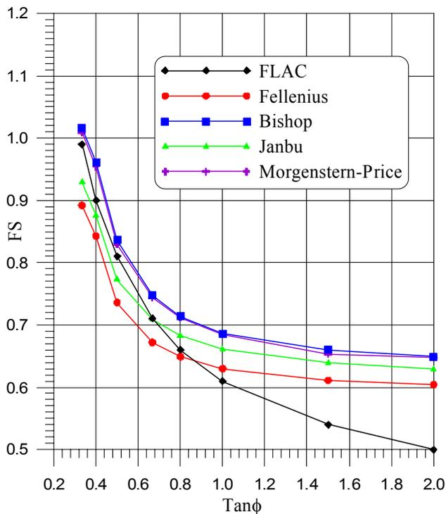
Figure 2. FS for embankment (height 25 m) consisting of two geological units for several sloping angles with SSR and LEM.
