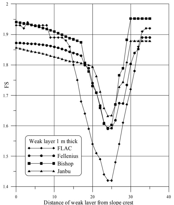
Figure 2. FS values for a 1.0 m thick weak layer.
