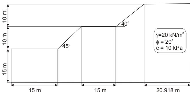
Figure 5. Benched slope case geometry.
