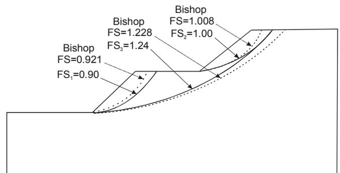
Figure 6. Several slip surfaces identified in benched slope by MSSR and LEM.
