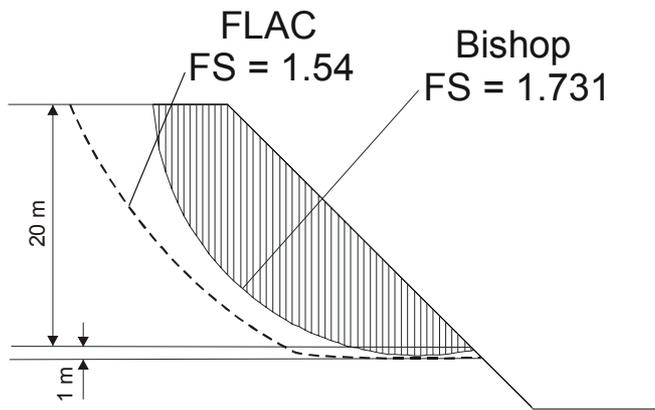
Figure 4. Critical slip surfaces identified by SSR and LEM.
