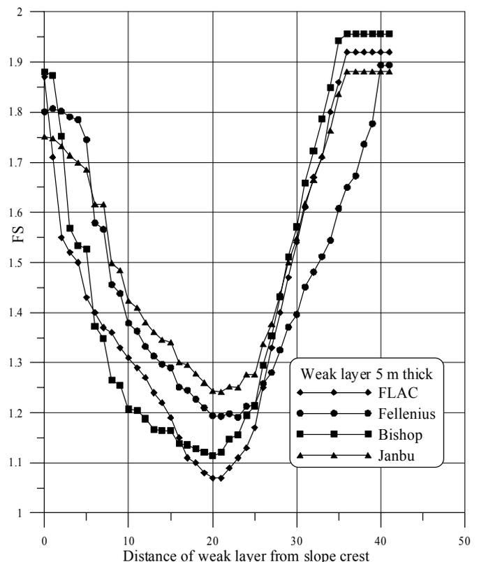
Figure 3. FS values for a 5.0 m thick weak layer.
