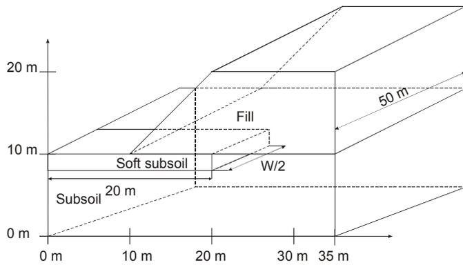
Figure 1. The details of modeled geometry.
