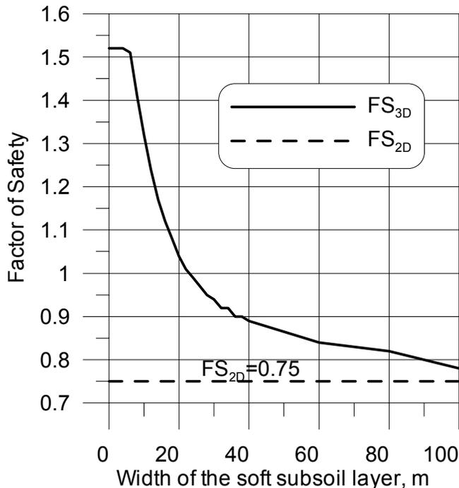
Figure 4. 2D and 3D FS values for several soft subsoil widths (thickness – 2 m).
