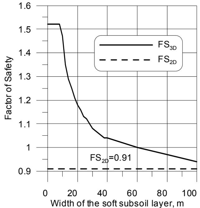
Figure 2. 2D and 3D FS values for several soft subsoil widths (thickness – 1 m).
