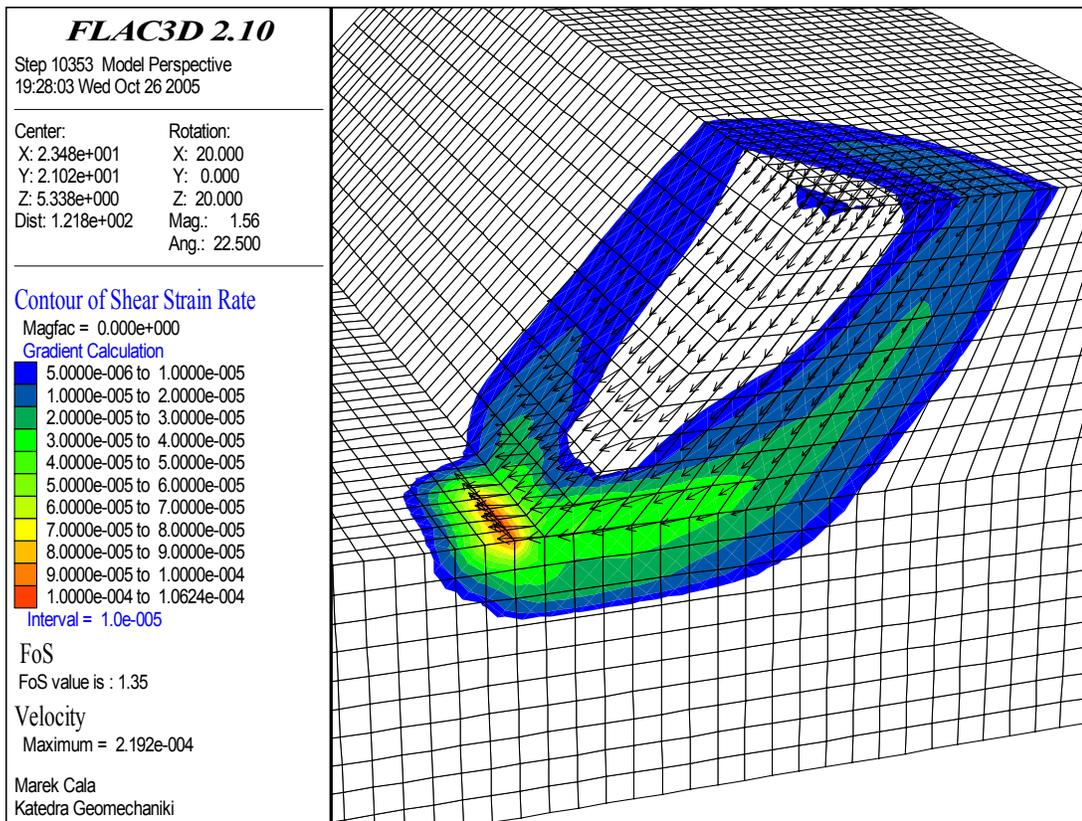
Figure 3.  $FLAC^{3D}$  model showing failure mode for the width of the subsoil  $W = 12$  m (thickness 1 m).
