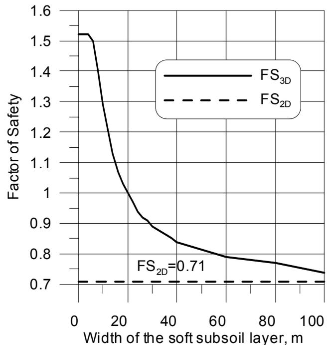
Figure 5. 2D and 3D FS values for several soft subsoil widths (thickness – 3 m).
