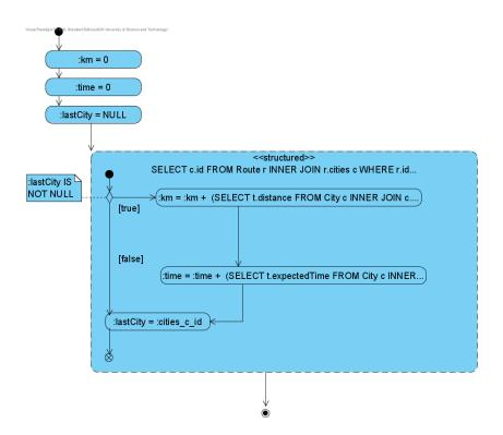
Fig. 5. Model of a procedure computing expected time and travel time of chosen route
