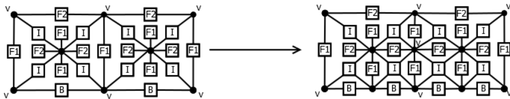
Figure 3.6: Production P_{enforceregularity} enforcing the 1-irregularity rule
