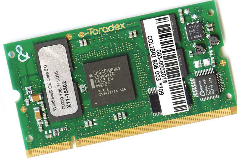
Fig. 2. The development kit of the PXA-270 microprocessor (real size: 67.6 x 36.7 x 5.2 mm)
