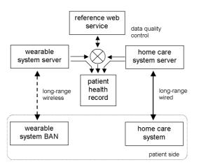
Fig. 2. Block diagram of two monitoring systems cooperation when measurement and interpretation competences are partly overlapping
