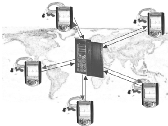
Fig. 1. The star-shaped architecture of adaptive ECG monitoring network
