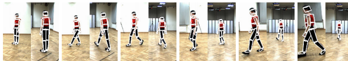
Fig. 2: Articulated 3D human body tracking in four camera setup. Shown are results in frames #0, 20, 40, 60, 80, 100. The left sub-images are seen from view 1, whereas the right ones are seen from view 2.
