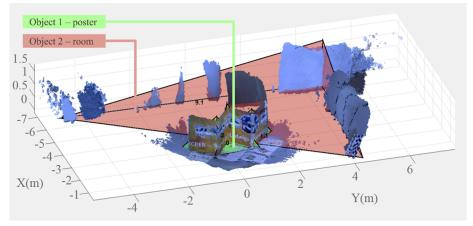
Fig. 1: Plane object-based high-level map representation on the point cloud reconstructed from 907 frames, represented by open TUM RGB-D dataset [20] (rgbd\_dataset\_freiburg3\_structure\_texture\_far).
