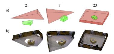
Fig. 7: Comparison of merging plane object-based high-level map representation using 6 DoF plane-to-plane correspondence (b) with merging point clouds reconstructed from color images and depth maps on each step using state-of-the-art ICP algorithm (a).
