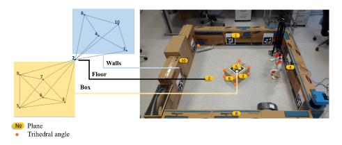
Fig. 3: The graph representing scene of the sequence 2 - a box in a simple room with four walls, which are observed by Nao humanoid robot.
