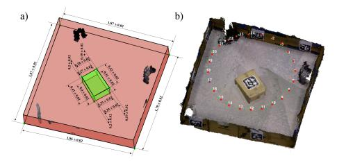
Fig. 8: Comparison of memory consumption of plane object-based high-level map representation for SLAM with point cloud. High-level map representation with estimated object sizes and errors (a). Ground truth trajectory (green points) in (b) has been determined using LMS 200 SICK laser scanner while the path (red points) has been estimated on the basis of visual odometry and our high level map representation.
