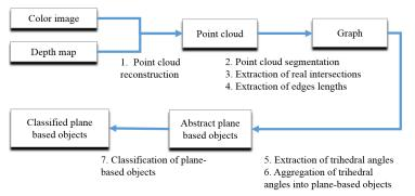
Fig. 2: Diagram representing transition from colored point cloud to classified plane object-based high-level map representation.
