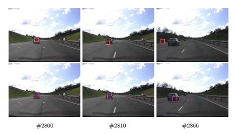
Fig. 4. The results of tracking using CamShift (top row) and particle filter (bottom row).
