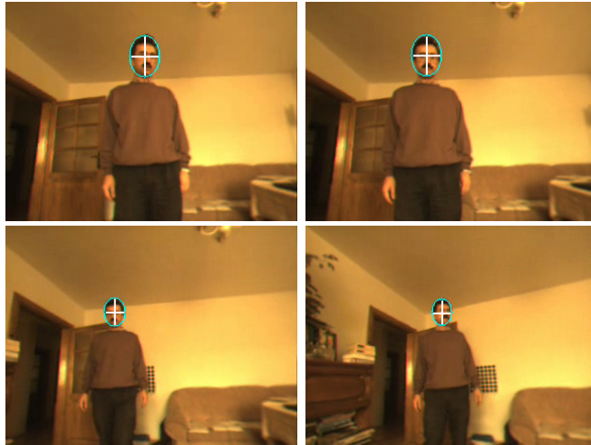
Fig. 2. Face tracking relying only upon a rotation of the moving camera (frames 1,35,390,600)
