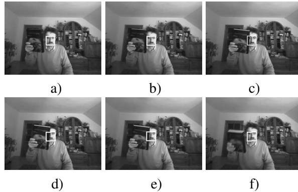
Figure 2. Particle swarm optimization based tracking of face undergoing temporal occlusions, frames #10 a), #15 b), #20 c), #25 d), #27 e), #28 f)
