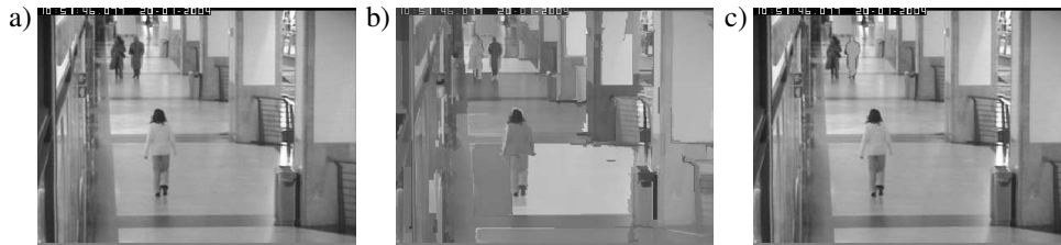
Figure 1. Image segmentation using pairwise region comparison and optical flow. Raw input image (a), segmented image (b), manually activated segment representing the object to be tracked (c).
