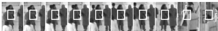
Fig. 2. Person tracking using swarm particle filter built on adaptive appearance models. Frames #888, #889, #899, #900, #909, #928, #929, #939, #1554, #1566
