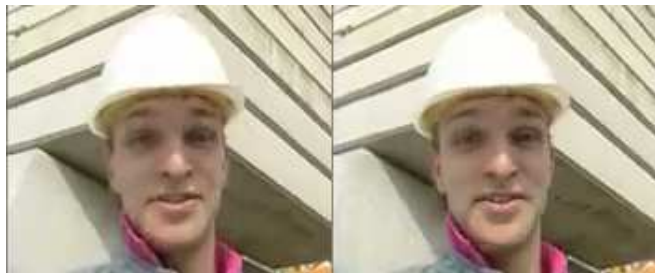
Fig. 1. Foreman frame #100 encoded with unmodified H.264 (left) and modified H.264 (right)
