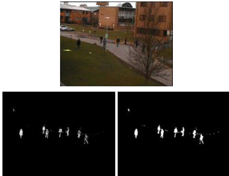
Figure 3: a) Input image. b) background probability image. c) Background refined by graph-cut
