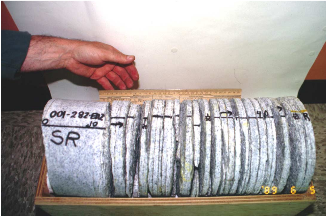
Figure 1.7: Disking of a 150 mm core of granite as a result of high in situ stresses.
