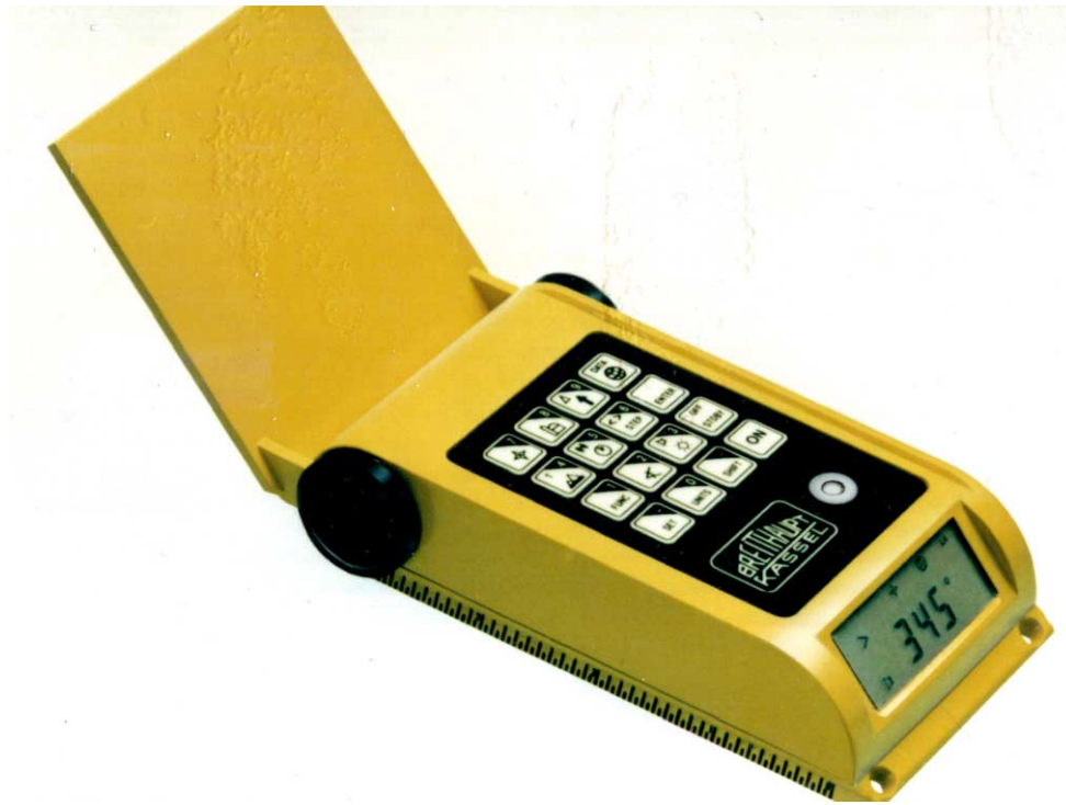
Figure 1.4: A Clar electronic geological compass manufactured by F.W. Breihapt in Germany.
