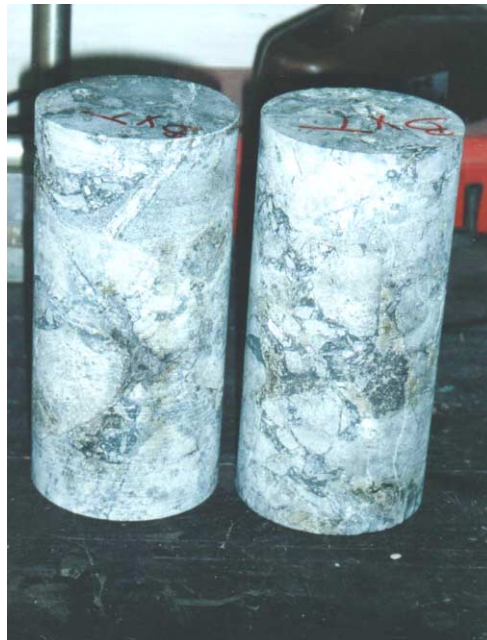
Fig. 11.19. 100 mm diameter by 200 mm long specimens of Braden Breccia from the El Teniente mine in Chile.
