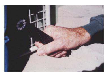
Figure 14.15: Hollow cable by Atlas Copco.
