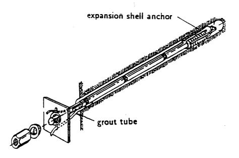
Figure 6.2: Mechanically anchored rockbolts of the type used on the Rio Grande project. These bolts were tensioned to 70% of their yield load upon installation and then, at a later stage, were re-tensioned and fully grouted.
