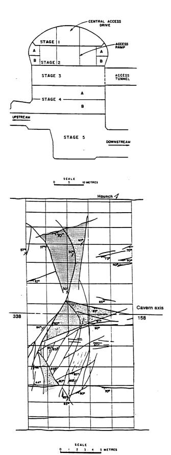
Figure 6.5: Cavern profile and excavation stages.
