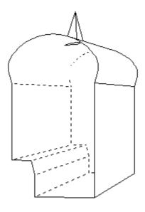
Figure 6.11: Perspective view of roof wedge in the Rig Grande cavern roof. The size of this wedge has been defined by setting the trace length of the 50/345 joint to 10 m.
