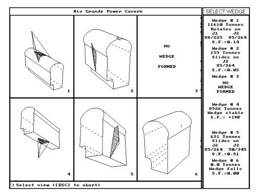
Figure 6.10: Perspective view of the wedges formed in the rock mass surrounding the Rio Grande power cavern.
