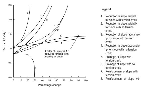
Figure 7.12: Evaluation of remedial options to increase the stability of the slope
