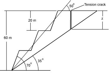
Figure 7.5: Geometry assumed for the two-dimensional analysis of the Sau Mau Ping Road slope.
