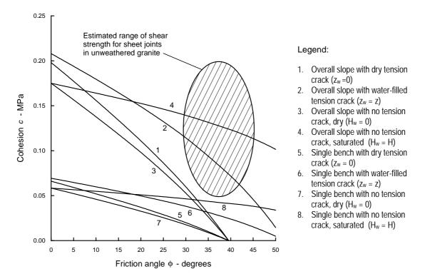
Figure 7.9: Comparison of the shear strength mobilised by failure under various conditions with the estimated shear strength available on sheet joints in unweathered granite.
