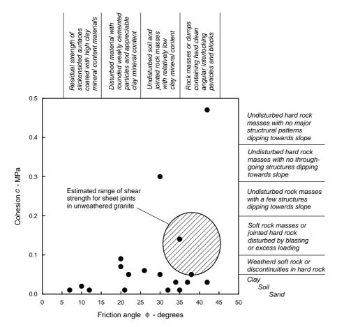
Figure 7.8: Relationship between friction angles and cohesive strengths mobilised at failure of slopes in various materials. The plotted points were obtained from published information from the back analysis of slope failures. (After Hoek and Bray 1974).
