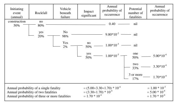
Figure 9.12: Event tree for a hypothetical example in which construction activities on the Argillite Cut are carried out for a period of six months while the highway is kept open.
