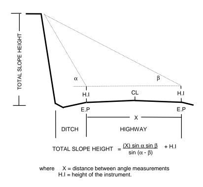
Figure 9.9: Measurement of slope height.
