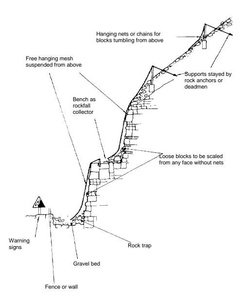
Figure 9.6: Rockfall control measures. After Fookes and Sweeney (1976).
