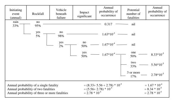
Figure 9.11: Event tree analysis of rockfalls in the Argillite Cut in British Columbia. (After Bunce, 1994)
