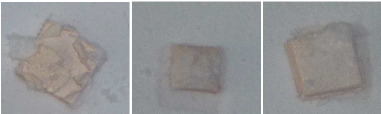
Fig. 5. Samples after ceramization in 1050°C (Samples A, B, C - from left to right hand side).
