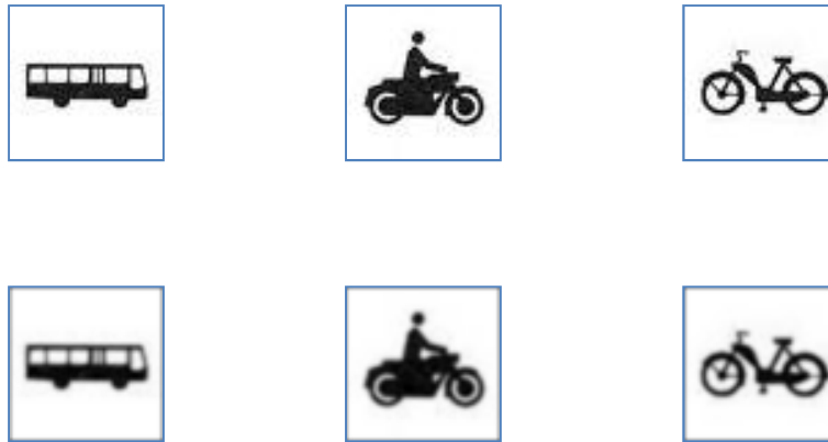
Fig. 1. Visualization of Standardizing Transform applied to the road sign pictograms. Original pictograms (upper row). After transformation (lower row).
