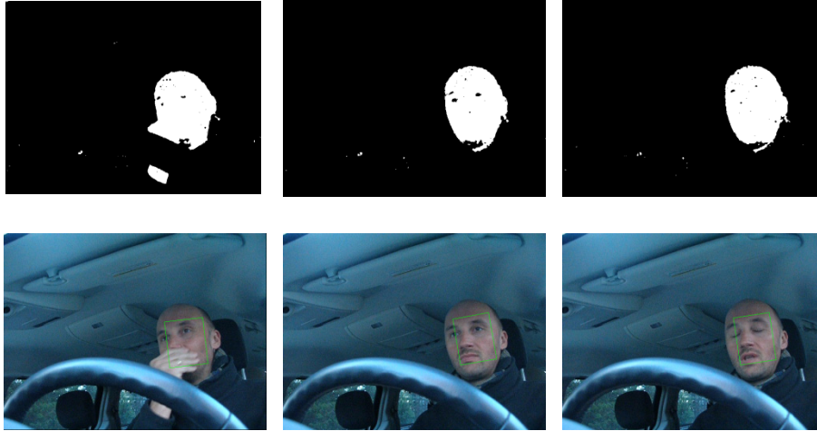
Fig. 5. Results of person head tracking in a driver's monitoring system. Detected pixels with an ensemble of three OC-SVMs (top row). Head orientation from the mean shift method (bottom).
