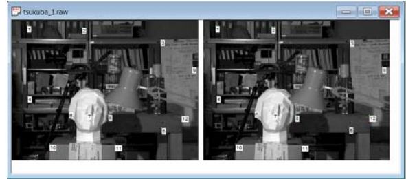
Figure 3. A stereo pair with manually selected points. These can be used to compute a reference epipolar geometry.
