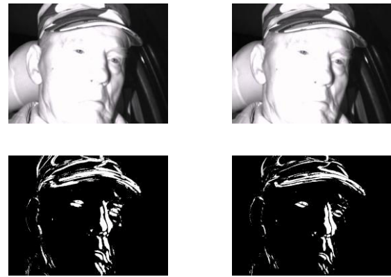
Figure 5. Eigenbackground subtraction. Test frames in upper row. Eigenbackground in lower row. White areas correspond to moving parts of the scenes.
