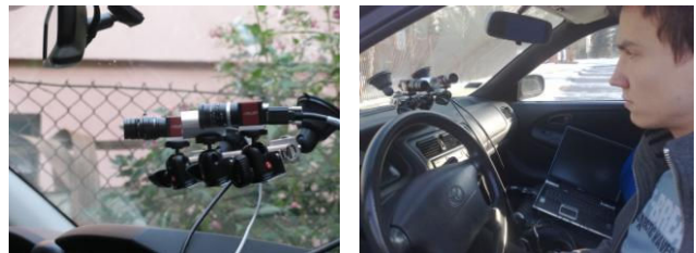
Figure 1. Presented system for driver's eye recognition mounted in the cars. The acquisition system contains two cameras, one for the visible and one for the NIR spectrum. NIR lighting is obtained with the external LED.
