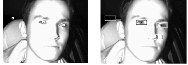
Figure 9. Example of eye detection in a test sequence. Left image contains all pupil candidates. Candidate eye regions which are fed to the HOSVD eye recognition module for final validation are shown in the right image.
