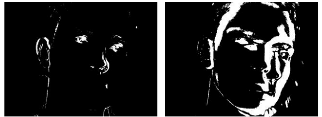
Figure 10. Moving parts of a driver detected with the eigenbackground subtraction method.
