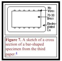
Kirkendall found a shrinkage of the brass core. Figure 8 shows the shift of each interfacehalf the total decrease in interface-to-interface distance. On the basis of the sample analysis described in the second paper, the interdiffusion coefficient was evaluated from these diffusion penetration profiles as
