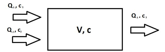
Assuming, that incoming fluxes with contamination started at certain moment of time t=0 and that  $Q_1+Q_2=Q_3$ , determine the concentration of contaminant in the system over time c(t). Our initial condition, is that  $c(t=0)=c_0$ .
