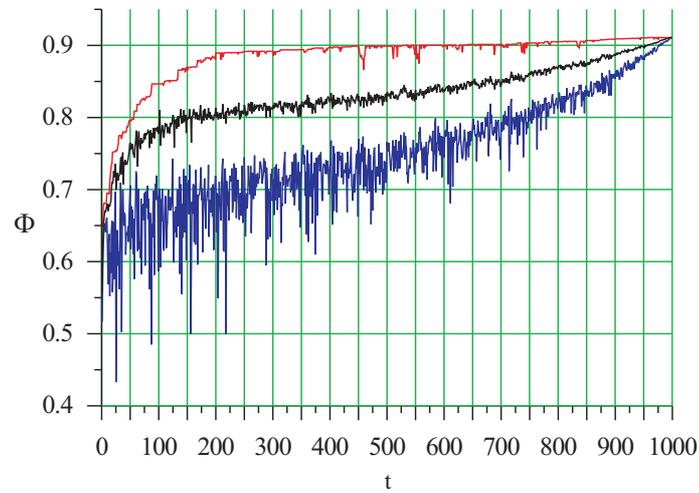
**Fig. 6.** Minimum (bottom line), average (middle line) and maximum (top line) value of the objective function for combined mechanisms  $M1$ ,  $M2$  and  $M3$  (the deterministic standard deviation modification, crowding and elitism)
