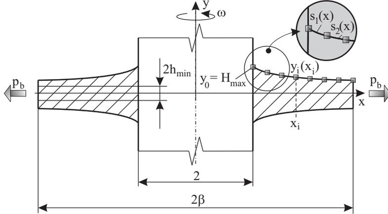
**Fig. 1.** Annular disc under consideration and its profile representation
