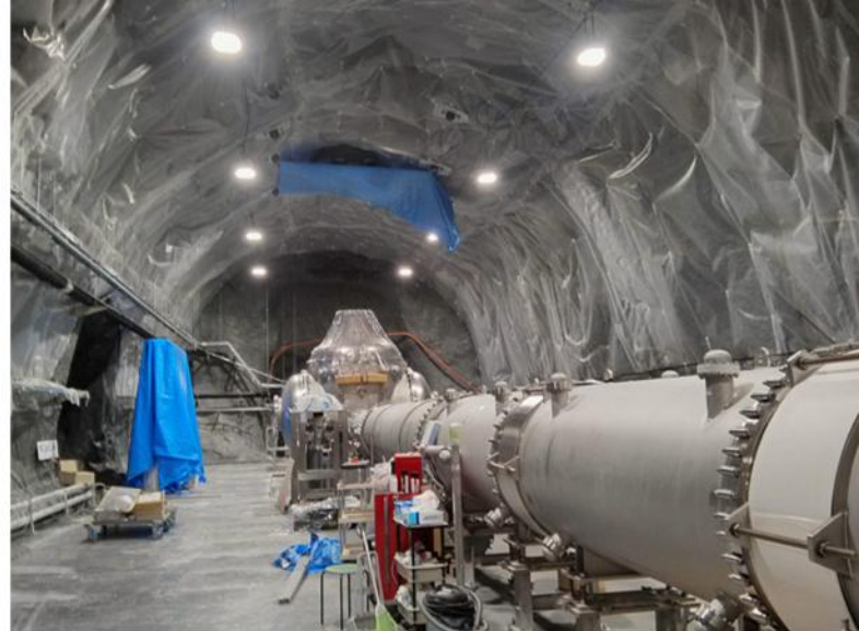
Japan's underground Kamioka Observatory houses the KAGRA gravitational wave detector, which should begin observations in 2018. This view shows one of the interferometer's arms. WIKIMEDIA COMMONS/CHRISTOPHER BERRY (UNIVERSITY OF BIRMINGHAM)
