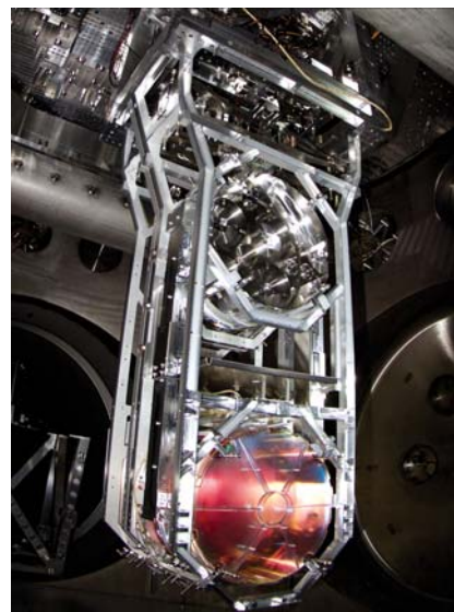
FIGURE 3. EACH MIRROR in LIGO's optical cavities sits at the end of a so-called quadruple pendulum. The 40 kg mirror (bottom) is not attached to the outside frame but hangs from the 40 kg silica cylinder above it by a set of fused silica fibers. The cylinder in turn hangs from a metal mass, which is hanging from yet another suspended metal mass. The system is designed to minimize thermal noise and passively dampen any environmental vibrations that get past LIGO's active seismic isolation system. (Courtesy of Caltech/MIT/LIGO Laboratory.)
