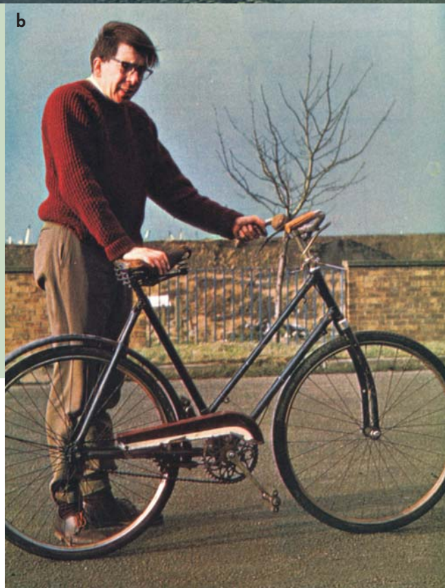
Figure 1. Unridable bicycles. David Jones is seen here with three of his experimental machines, two of which turned out to be rideable after all. (a) At the top of this page is URB I, with its extra counter-rotating front wheel that tests the gyroscopic theories of bicycle stability. (b) At left is URB III, whose reversed front forks give it great stability when pushed and released riderless. (c) URB IV (immediately above) has its front wheel mounted ahead of the usual position and comes nearest to being “unrideable.”
