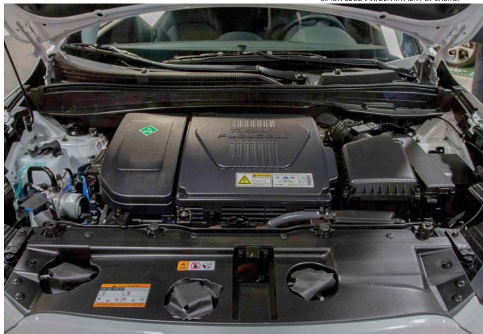
THE HYUNDAI TUCSON, POWERED BY A HYDROGEN FUEL CELL, emits only water. It is one of three fuel-cell car models for sale in California.
