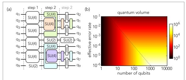
**Figure 2.** (a) Example quantum circuit with two circuit steps. Step 2 requires different connectivity and would lead to an increased gate count on quantum hardware with only nearest neighbor interactions. This is illustrated to the right of step 2. (b) Quantum volume as a function of the effective error rate  $\epsilon_{\rm eff}$  and the physical number of qubits N. For simplicity, we assume that for a given  $\epsilon_{\rm eff}$   $V_{\rm Q}$  stays constant for d < N.
