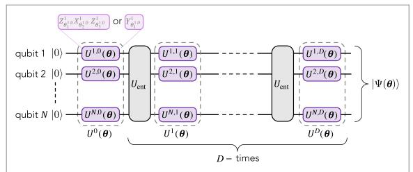
Figure 4. Heuristic preparation of trial states for the variational quantum eigensolver based on single-qubit gates  $U(\theta)$  interleaved by entangling operations  $U_{\rm ent}$  as described in the text.
