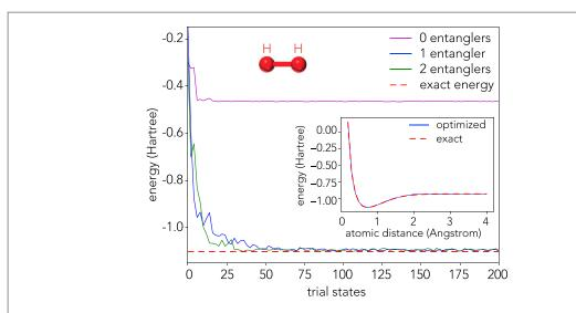
**Figure 5.** Quantum simulation of the hydrogen molecule on an ideal quantum simulator. At the equilibrium geometry and no entangler block in the circuit, the energy converges to a state with an energy that is about 50% too high. With two or more entanglers, the exact energy is obtained. The inset shows the entire dissociation profile for a hydrogen molecule calculated with four entangling steps.
