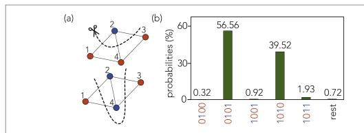
**Figure 6.** (a) Two different cuts for a MaxCut instance with four vertices. The lower cut has a larger cumulated weight and represents the partitioning that solves the problem. (b) Solution of the problem using the VQE with heuristic trial-states and a depth D=3 circuit.
