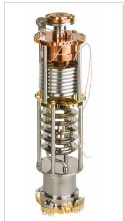
Modern dilution unit with silver heat exchanger
