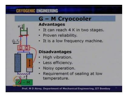
And advantages are it can reach 4 Kelvin in two stages. It has got proven reliability for quite sometimes. It is a low frequency machine as you know, and therefore, the vibrations are at low frequency here.
