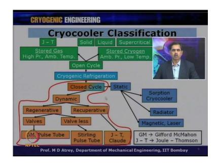
Now, coming to cryocooler classification. If I see cryocooler classification, the cryocoolers can be classified based on how you get cryogenic refrigeration. So, this is the most important thing. So, I can get cryogenic refrigeration in two ways: one is by open cycle, the other one is by closed cycle. Please understand this slide very importantly now.
