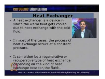
So, a heat exchanger is a device in which the warm fluid gets cooled due to heat exchange with cold fluid, as you know this. In most of the cases, the process of heat exchange occurs at a constant pressure. It can either be a regenerative heat exchanger or recuperative heat exchanger depending on the kind of heat exchange between the fluids. So, you know the basics of heat exchanger, where warm and cold fluid exchange heat.
