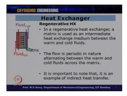
Now, let us see regenerative heat exchanger, and in the regenerative heat exchanger, a matrix is used as an intermediate heat exchange medium between the warm and cold
