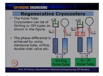
Now, this pulse tube Cryocooler can be with valve or without valve, which means; they can be of Stirling type pulse tube cooler; which is without valve, and also they could of G-M type pulse tube cooler; which means there is a valve elements between the compressor and expander. This is called as Stirling type pulse tube cooler. This is called as G-M type pulse tube cooler. As I said, this is the high frequency machine. This could be a low frequency machine.
