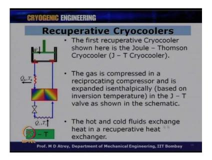
Now, in the recuperative case, if I want to see now recuperative cryocooler, you have got a compressor, heat exchangers and Joule Thomson expansion. So, this is a Joule Thomson cryocooler which uses a recuperative heat exchanger.
