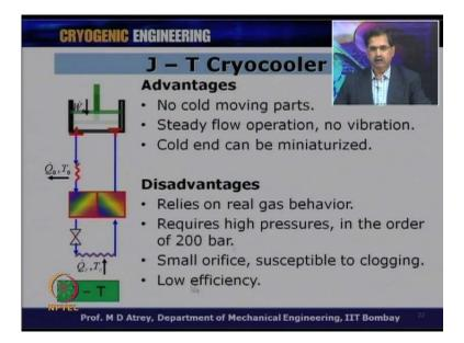
So, these are different highlights of J-T Cryocooler, the advantages are nothing moving on the cold sides. So, no cold moving part. Steady flow operation, and therefore, no vibration. You have got a high pressure line and low pressure line. Nothing oscillating. No pressures are oscillating. There is no oscillating flow in this case, and therefore, no vibration. The cold end can be miniaturized.
