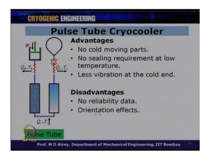
The advantages are: no cold moving parts as you know here, nothing is moving, no sealing requirement because there is no displacer here, there is no sealing requirement at low temperature which is very much required in G-M coolers, less vibration at the cold end because there is no mechanical displacer at this point.
