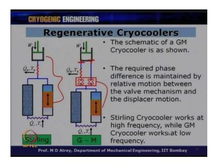
Now, the next cryocooler what we call is a Gifford McMahon cryocooler, and what you can see here, there is a only one line; high pressure, low pressure was travelling from this, while here we have got a high pressure line and a low pressure line; separate line because the compressor kind of compressor used here will have two valves, inbuilt valves over here which are actually direction dependent valves.
