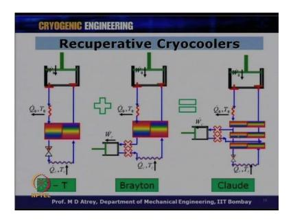
Now, you can (()) the second cycle which is Brayton cycle. Instead of having this valve, we can have an expander which is a moving expander, and it has got an inlet valve and exhaust valve. And depending on this expansion, this will produce work output over here. This will not produce work output here, but this will work output, and therefore, what we call is a Brayton cycle.
