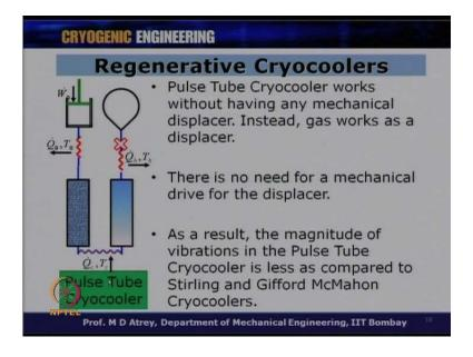
In addition to this Stirling and G-M, what we have is also pulse tube cryocooler. So, what you can see in pulse tube cryocooler is, there is no displacer and the expander here. There is no mechanical displacer over here, and therefore, we do not require a drive for this also. In earlier two case, is because the displacer is moving, we will require a drive mechanism for this displacer motion also.
