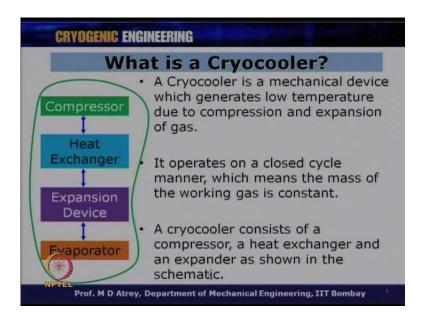
Now, let us see, what is a cryocooler. So, Cryocooler is a mechanical device which generates low temperature due to compression and expansion of gas. Simple thing. It is like any other domestic refrigerator. A cryocooler actually is nothing but a refrigerator which gives you cryogenic temperature, which generates temperature in cryogenic range, and actually some people will call it Cryogenic Refrigerator also.
