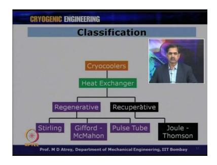
Now, let us come to the classification of cryocoolers, and as I said earlier, the cryocoolers are classified based on the kind of heat exchanger it uses. So, every cryocooler will have some kind of heat exchanger, and every heat exchanger, the heat exchanger could be of two types; a Regenerative type and Recuperative type. I will talk about this in the next slides.
