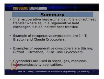
In a recuperative heat exchanger, direct heat transfer, whereas, in regenerative heat exchanger, it is indirect heat transfer.
