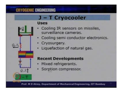
Now, let us go through each cryocooler and just see advantages and disadvantages of various cryocooler. So, a J-T Cryocooler is used for cooling infrared sensors on missiles, surveillance cameras. It can be used for cooling semiconductor electronics and also recently, it is being used for cryosurgery because the high pressure gas just goes in, it
