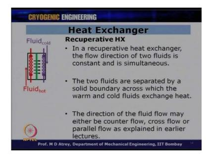
Now, in a recuperative heat exchanger, the flow direction of two fluid is constant and is simultaneous. So, you can see that, this is a recuperative type of heat exchanger where
