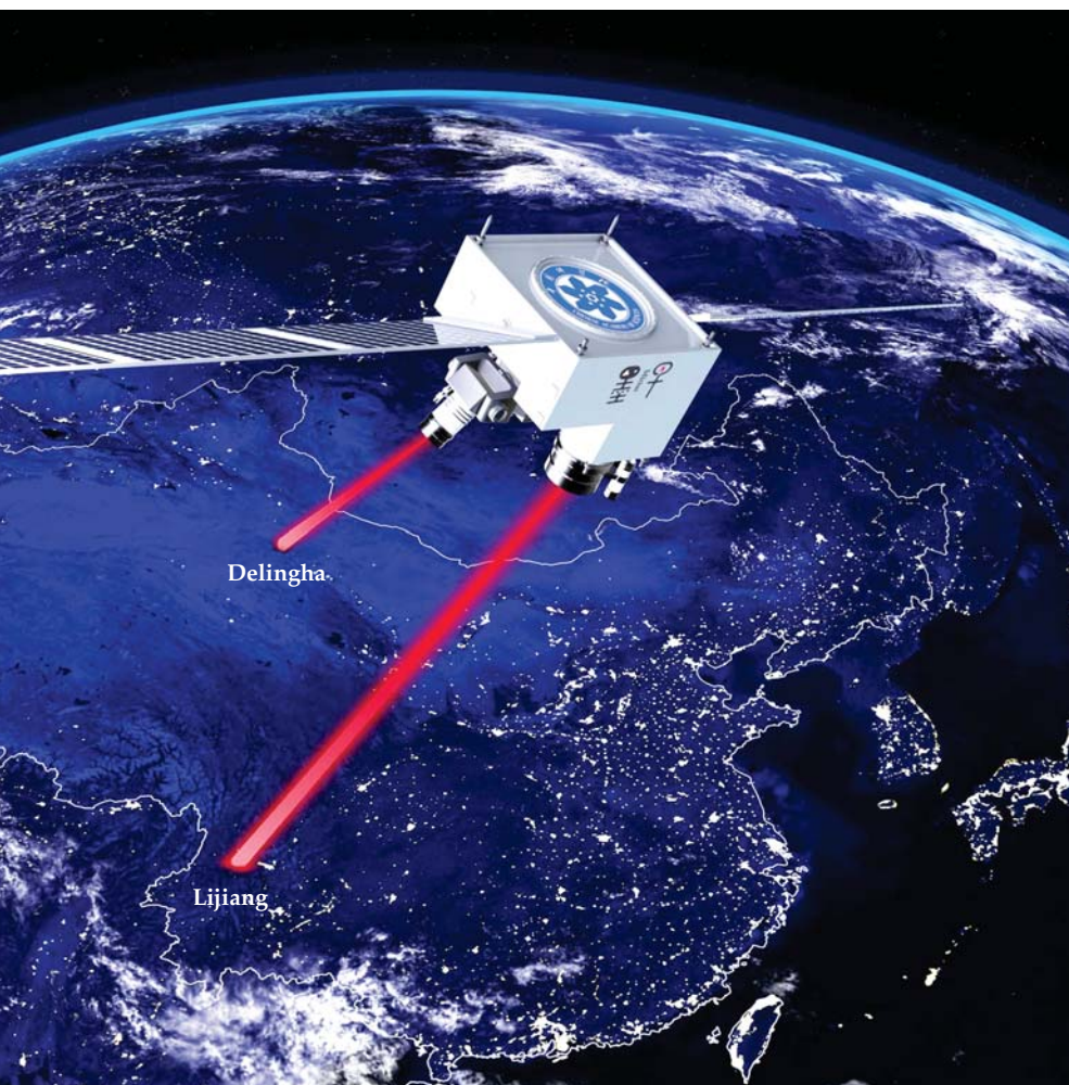
FIGURE 1. THE QUANTUM SCIENCE SATELLITE , nicknamed Micius , successfully beamed polarization-entangled photons from low-Earth orbit to two ground stations 1200 km apart in Delingha and Lijiang, China. Such satellite-based entanglement distribution could provide the basis for a highly secure quantum communications network. (Illustration courtesy of Jian-Wei Pan.)
