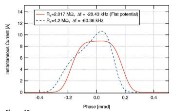
**Figure 15** Equilibrium longitudinal bunch density distribution for two different settings of the HC system in the MAX IV 3 GeV ring.
