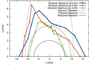
**Figure 6**Dynamic aperture at the centre of the long straight section in the bare lattice of the MAX IV 3 GeV storage ring (Leemann, 2012*d*). Tracking was performed with *Tracy-3* in 6D for one synchrotron period. For comparison, the vacuum chamber and physical aperture (projection of vacuum chamber to the track point) are also indicated in the plot.
