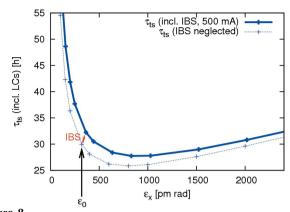
Figure 8 Touschek lifetime as a function of equilibrium emittance assuming the bare lattice emittance could be adjusted freely while keeping the energy spread constant (Leemann, 2012d). The overall MA has been set to 4.5% while the vertical emittance is adjusted to 8 pm rad. The effect of Landau cavities (LCs) is included. The equilibrium emittance of the MAX IV 3 GeV storage ring bare lattice  $\varepsilon_0$  = 328 pm rad is indicated.
