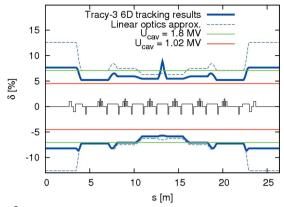
**Figure 9**Lattice momentum acceptance for one achromat of the MAX IV 3 GeV storage ring (Leemann, 2012d). A bare lattice with actual vacuum chamber apertures has been used. The solid blue line shows lattice MA from 6D tracking with *Tracy-3*. For comparison, the RF acceptance is shown as well: cavities at maximum voltage 1.8 MV (7.1% RF acceptance) and at 1.0 MV (4.5% RF acceptance).
