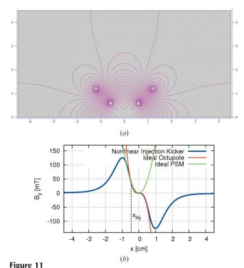
Upper half geometry (top) and resulting field profile in the midplane (bottom) of a BESSY-type non-linear injection kicker adapted to the MAX IV 3 GeV storage ring (Leemann & Dallin, 2013). Note that the resulting field around the centre is similar to an octupole.
