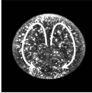
**Figure 2.5:** A snapshot of a bounce (at a maximum of trajectory) of a 5 cSt silicone oil droplet on a high viscous bath that oscillates at 50 Hz and at an acceleration  $\Gamma = 2.5$ . The internal flows are revealed by fluorescent microspheres.
