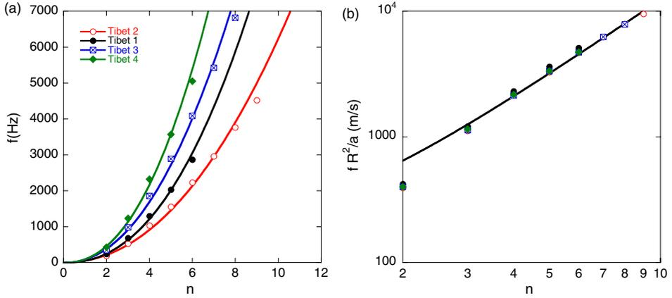
**Figure 4.** (a) Measurements of the resonant frequencies of the different deformation modes  $n$  for the 4 different Tibetan bowls. (b) Characteristic speed  $fR^2/a$  as a function of deformation mode  $n$  for the 4 different bowls. Data are fit by a power 2 curve indicating that  $f_n \propto n^2 a/R^2$ , consistent with equation (6).
