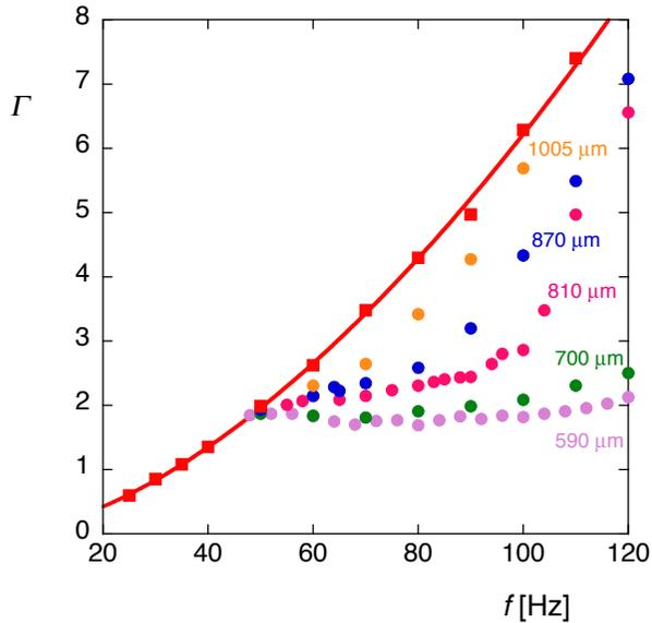
**Figure 4.4:** The acceleration threshold  $\Gamma_{PDB}$  (transition from a mode (1,1) to a mode (2,2)) as a function of the frequency for several droplet diameters which are indicated on the figure. The Faraday threshold measurements are represented by red square symbols which are fitted, in red, by a power 5/3 of the frequency.
