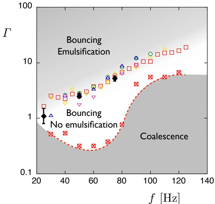
**Figure 2.18:** Bouncing threshold acceleration  $\Gamma_b$  ( $\boxtimes$ ) and emulsion threshold acceleration  $\Gamma_e$  ( $\square$ ,  $\diamond$ ,  $\triangle$ ,  $\circ$ ,  $\nabla$ ) as a function of the forcing frequency  $f$ . Symbols correspond to various sizes of the compound drop, as detailed in Table 2.2. Black diamonds are explained in Fig. 2.22 (cf. text).
