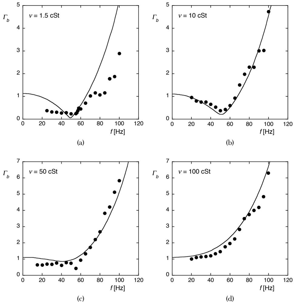
**Figure 2.9:** a) Acceleration threshold  $\Gamma_b$  required for the bouncing for various drop viscosities: (a)  $\nu = 1.5$  cSt, (b)  $\nu = 10$  cSt, (c)  $\nu = 50$  cSt and (d)  $\nu = 100$  cSt. The solid line corresponds to the model prediction, with coefficients  $c_{L_2} = 17.5$ ,  $c_K = 0.1$ ,  $c_\sigma = 16\pi/5$  and  $c_D = 3$  (cf. Section 2.3).
