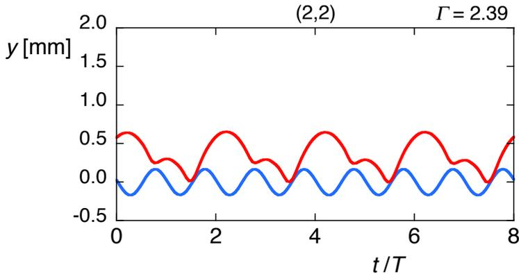
**Figure 4.8:** A droplet of diameter  $D = 690 \mu\text{m}$  is walking in a bouncing mode  $(2, 2)$  on a liquid bath oscillating at  $58 \text{ Hz}$  at  $\Gamma = 2.40$  (just below the Faraday threshold). Both liquids are  $20 \text{ cSt}$  silicone oil. The vertical position  $y$  of the droplet (in red) and bath (in blue) are reported as a function of the normalized time  $t/T$ .
