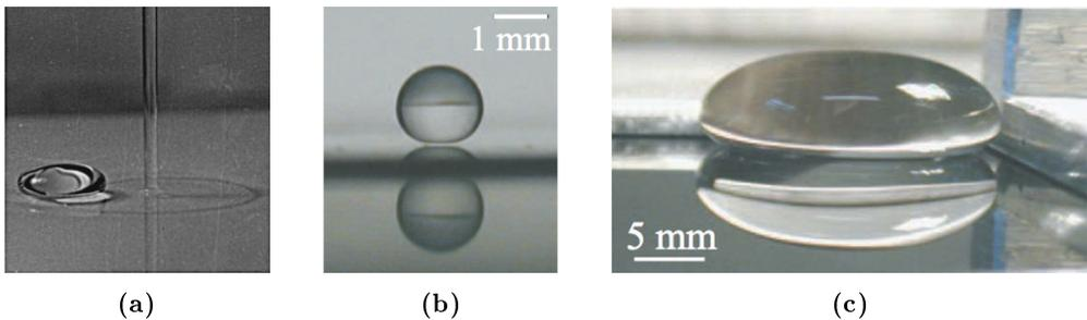
**Figure 1.2:** a) A water droplet of diameter 1.6 cm levitating due to a hydraulic jump (from [19]). b-c) Water drops deposited on a solid silicon surface maintained at a temperature of 200° C (from [21]).
