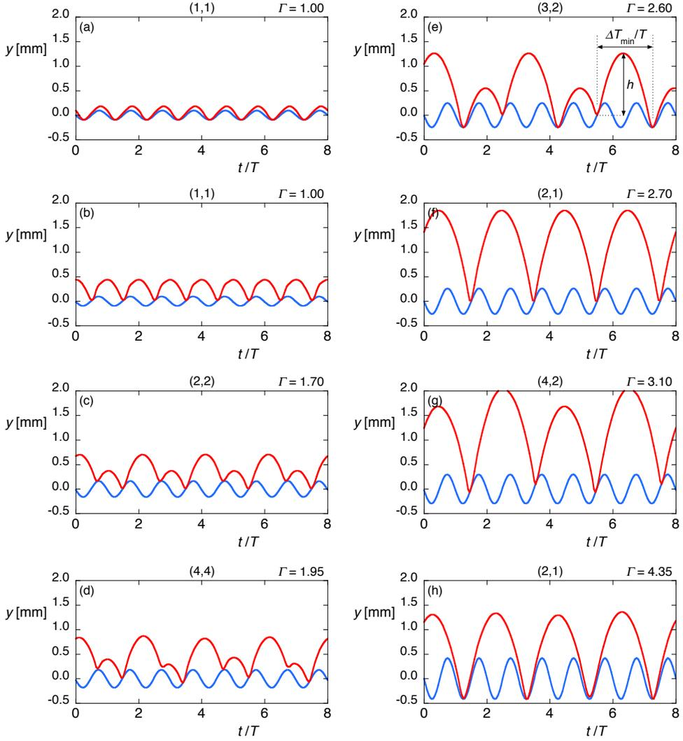
**Figure 3.5:** Experimental trajectories of a 20 cSt silicone oil droplet of diameter  $D = 890 \mu\text{m}$  bouncing on a bath oscillating at a frequency of 50 Hz for various accelerations  $\Gamma$ . The bouncing mode  $(p, q)$  and the forcing acceleration  $\Gamma$  are indicated on each figure. The time interval  $\Delta T_{\min}$  between two successive bounces and the bouncing heights  $h$  that are measured on each trajectory are illustrated on figure (e).
