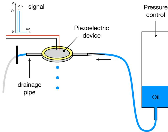
**Figure C.1:** Schematic illustration of the droplet dispenser.
