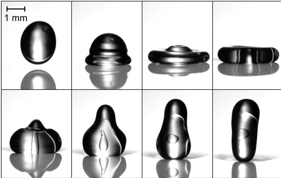
**Figure 2.19:** A compound drop ( $\Delta$  in Table 2.2) bounces on a liquid surface vibrating sinusoidally at  $f = 50$  Hz and  $\Gamma = 4.4$ . The convergence of capillary waves on the top of the drop pushes the oil layer inwards. The water-oil interface pinches off and a tiny oil droplet is released into the water core.
