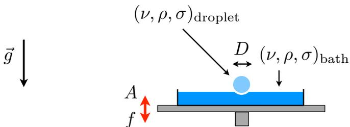
**Figure 1.10:** Schematic illustration of a droplet bouncing on a vibrating liquid bath. Relevant parameters are the gravity acceleration  $g$ , the droplet diameter  $D$ , the viscosity  $\nu$ , the density  $\rho$  and the surface tension  $\sigma$  for the bath and the droplet, the amplitude  $A$  and the frequency  $f$  of the oscillating plate.
