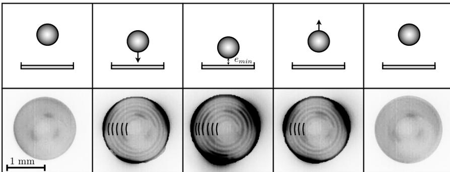
**Figure 2.10:** A droplet bounce - Successive snapshots of interference fringes (accentuated with black arcs) made by a bouncing droplet. The snapshots are separated by 8 ms. The number of observed fringes is directly related to the film thickness which varies between 100 nm and 10  $\mu\text{m}$ . An increasing number of fringes is visible when the droplet lands and squeezes the air film (until the third column), then the number of fringes decreases as the droplet lifts off.
