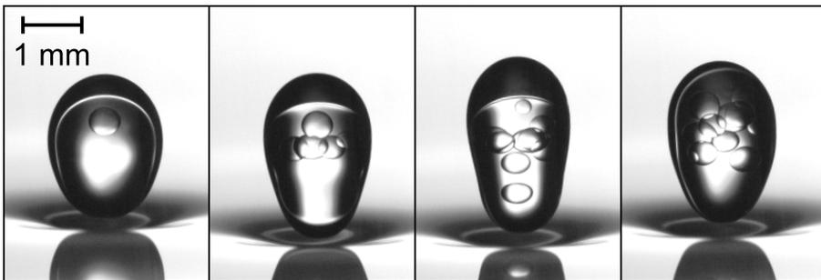
**Figure 2.20:** Each time the droplet impacts the bath with sufficiently high velocity, an additional oil droplet is injected into the inner water drop, progressively creating a double emulsion of oil droplets into a water drop surrounded by an oil shell. The four snapshots represent the same compound drop after 5, 20, 34 and 51 bounces.
