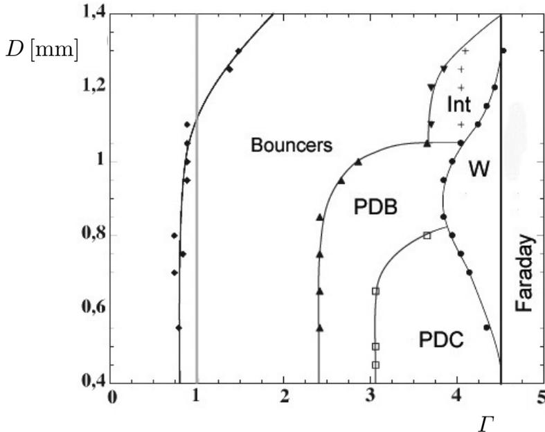
**Figure 1.7:** Bouncing droplets, on a 50 Hz oscillating bath, experience different bouncing modes which depend on their diameter  $D$  and the bath acceleration  $\Gamma$ . The liquid used for droplets and the bath is 50 cSt silicone oil. Region “Bouncers” corresponds to simple droplet bouncing, “PDB” to period doubling bouncing, “PDC” to a transition to chaos, “Int” to an intermittent behavior and “W” is the walker region, situated just below the Faraday instability region (from [25]).
