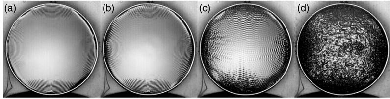
**Figure 7.** Evolution of the surface waves in Tibet 1 bowl filled with water and excited with a frequency  $f = 188$  Hz corresponding to its fundamental mode (2,0). The amplitude of deformation is increasing from left to right: (a)  $\Gamma = 1.8$ , (b)  $\Gamma = 2.8$ , (c)  $\Gamma = 6.2$ , (d)  $\Gamma = 16.2$ .
