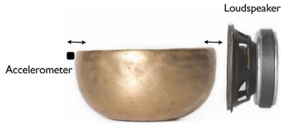
**Figure 6.** Experimental setup. The bowl deformation is excited by a loudspeaker emitting sound at a frequency corresponding to a particular vibrational mode of the bowl. The deformation of the bowl is measured by an accelerometer glued to the bowl's outer wall at the height of the liquid surface.
