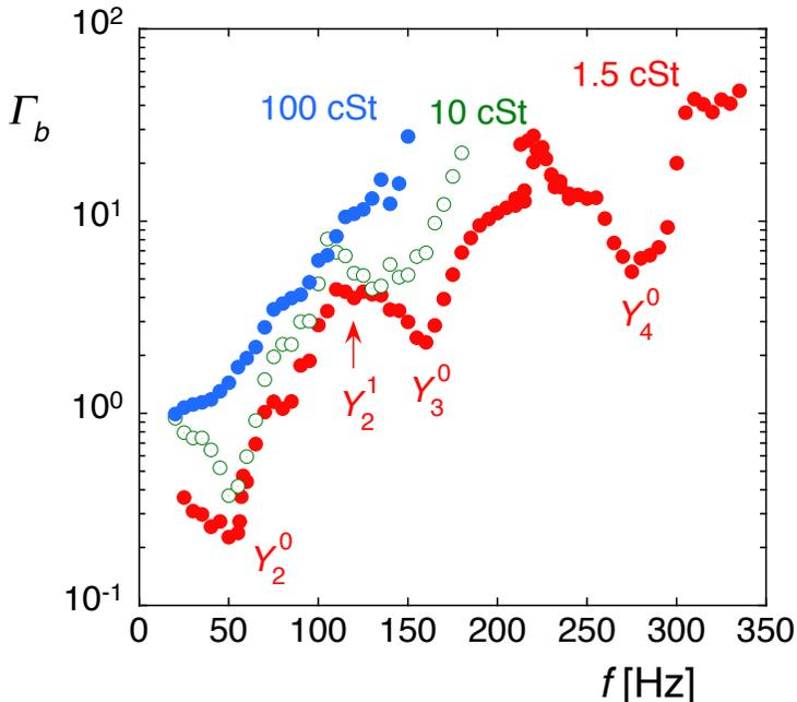
**Figure 2.1:** Evolution of the bouncing threshold acceleration  $\Gamma_b$  with respect to the forcing frequency. The red bullets ( $\bullet$ ), green circles ( $\odot$ ) and blue bullets ( $\bullet$ ) correspond to droplets with viscosity  $\nu = 1.5, 10$  and  $100$  cSt respectively, for a constant diameter  $D = 1.53$  mm. Depending on the forcing frequency, various modes are observed that are related to spherical harmonics  $Y_\ell^m$ .
