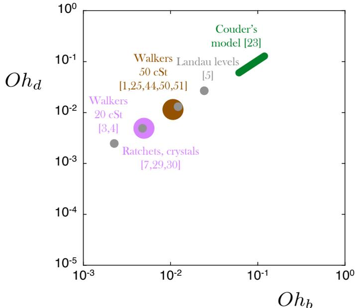
**Figure 1.11:** A selection of relevant works on bouncing droplets are plotted as a function of both Ohnesorge parameters  $Oh_d$  and  $Oh_b$  of the experiments. These represent the relative damping of the oscillations on the droplet and on the bath.
