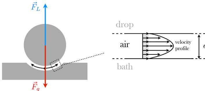
**Figure 1.1:** The air film between a floating droplet and a liquid bath is squeezed and drains out. In reaction, the air film of decreasing thickness  $e$  generates a lubrication force  $F_L$  that balances the droplet weight  $F_g$ . The airflow dynamics is a Poiseuille flow with a speed limit at boundaries which can be non negligible and change its shape.
