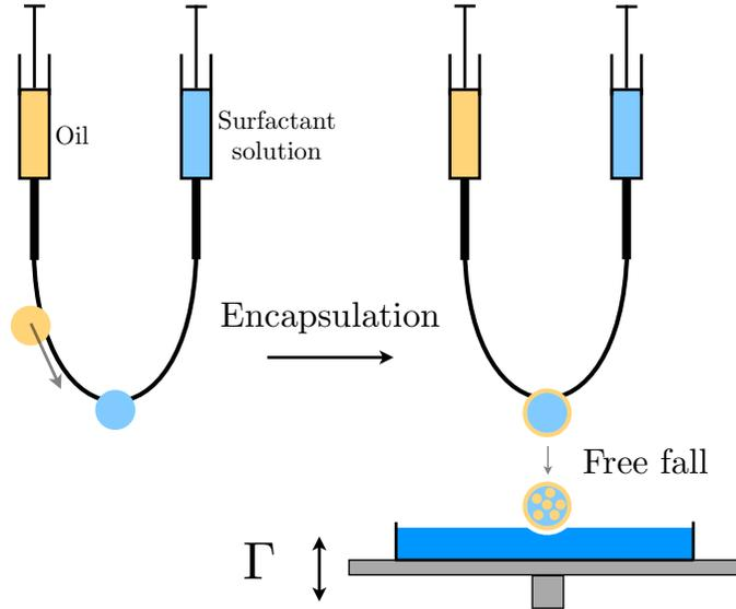
**Figure 2.17:** The compound drop is created by using two syringes connected by their ends by a thin copper wire. A water and an oil drop are respectively released from each syringe, they slide along the fiber and stop at the lowest point where they eventually merge. The compound drop detaches itself from the fiber and falls onto the oscillating liquid bath.
