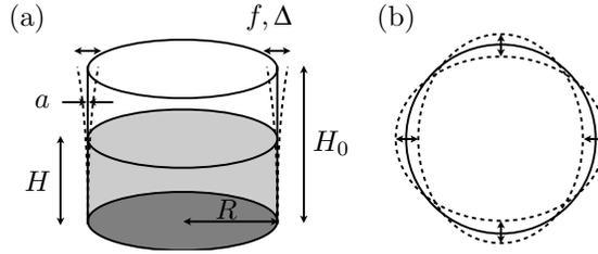
**Figure 2.** (a) Schematic illustration of a vibrating vessel filled with liquid. Relevant parameters are the height  $H_0$  and the radius  $R$  of the vessel, the thickness of the rim  $a$ , the liquid level  $H$ , the frequency  $f$  and the amplitude  $\Delta$  of the oscillating rim. (b) Top view of a vibrating vessel in its fundamental mode (2,0), characterized by its 4 nodes and 4 antinodes.
