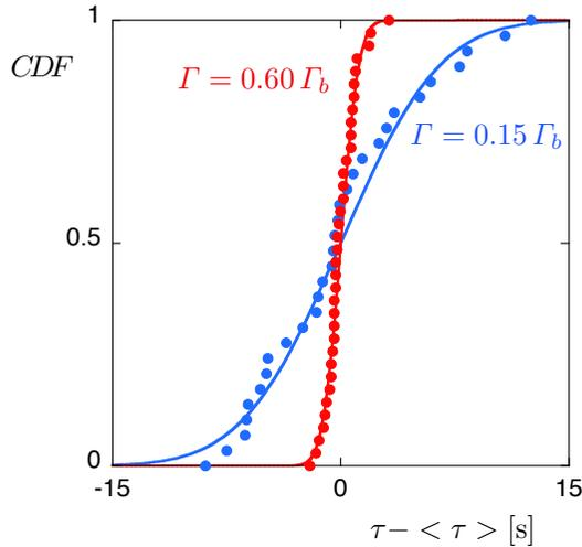
**Figure 2.11:** Cumulative Distribution Function  $CDF$  of the normalized lifetime of the bouncing droplets of diameter 1.68 mm ( $f = 75$  Hz,  $\nu = 10$  cSt) at various forcing accelerations (blue  $\bullet$ )  $\Gamma = 0.45$  ( $\Gamma = 0.15 \Gamma_b$ ), (red  $\bullet$ )  $\Gamma = 1.8$  ( $\Gamma = 0.6 \Gamma_b$ ). The lines represent fitted cumulative distributions function for Gaussian distribution which is typical of an aging process.
