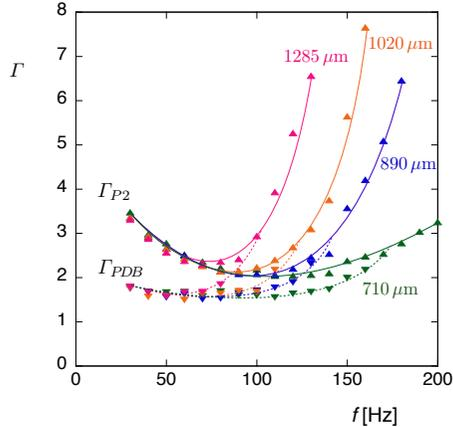
Fig. P.2: The transition accelerations  $\Gamma_{PDB}$  ( $\blacktriangledown$  symbol) and  $\Gamma_{P2}$  ( $\blacktriangle$  symbol) are measured for 4 different droplets which sizes are  $D_{\text{green}} = 710 \mu\text{m}$ ,  $D_{\text{blue}} = 890 \mu\text{m}$ ,  $D_{\text{orange}} = 1020 \mu\text{m}$ ,  $D_{\text{pink}} = 1285 \mu\text{m}$ . Diameters are indicated on the figure. The plain and dashed lines are guides for the eyes.
