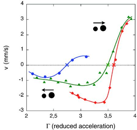
Fig. 2: The velocity of 3 couples of droplets as a function of  $\Gamma$ . The dots correspond to a couple of bound drops with  $D_1 = 0.87$  mm and  $D_2 = 0.96$  mm, the triangles to  $D_1 = 1$  mm and  $D_2 = 1.12$  mm and the rhombs to  $D_1 = 1.03$  mm and  $D_2 = 1.23$  mm. The continuous curves are simple interpolations. The crosses correspond to the reversal threshold  $\Gamma_1$ .
