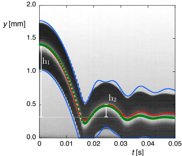
**Figure 3.8:** Zoom on the spatio-temporal of Fig. 3.2. The measurements of the center of mass are represented by black dots. The simulation of a falling spring system, from a height of  $h_1 = 1.1$  mm, with parameters  $k = 0.072$  N/m and  $\xi = 0.25$ , is represented by blue and red lines. The central red line is the trajectory of the center of mass and both outer blue lines are the trajectories of the masses  $m_1$  and  $m_2$ .
