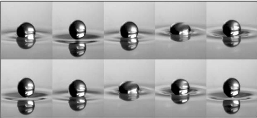
**Figure 1.3:** A drop of about 1 mm of diameter bounces on a liquid surface oscillating at 80 Hz together with an amplitude sufficient for the bouncing to occur. Drop and bath are made of silicone oil of viscosity 50 cSt.
