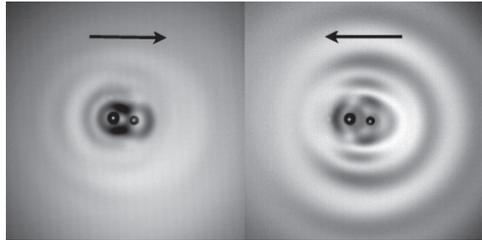
Fig. 4: Two top views of the same ratchet. Left: below  $\Gamma_1$  the larger drop emits a wave of larger amplitude. Thus the bound state propagates to the right. Right: over  $\Gamma_1$ , the smaller droplet has undergone a period doubling and emits a Faraday wave of larger amplitude: the bound state propagates to the left.
