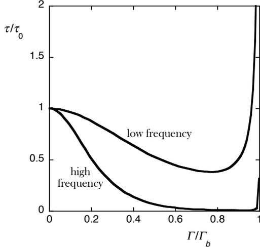
**Figure 2.15:** Schematic illustration of the normalized lifetime  $\tau/\tau_0$  as a function of  $\Gamma/\Gamma_b$ , according to the bouncing model [53] for a low frequency ( $f \rightarrow 0$  Hz) and a high frequency ( $f \sim 100$  Hz). Curves corresponding to the intermediate frequencies are of the same shape and are located in between these two curves.
