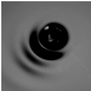
Fig. P.1: Top view of a droplet of several millimeter bouncing on an oscillating liquid bath at 100 Hz. The two liquids are made of 100 cSt silicone oil. This droplet is moving towards the top right corner [Credit: S. Protière]. It exhibits the characteristics of two self-propelled modes: the ratchet and the roller [7,47].
