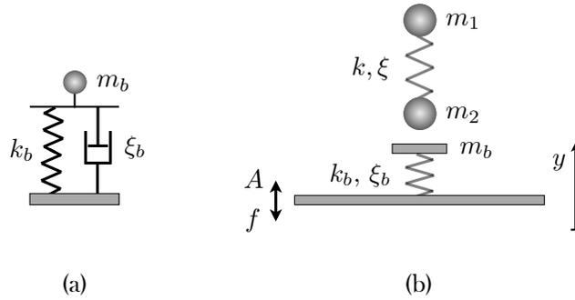
Fig. P.3: (a) The bath is modeled by a mass  $m_b$  linked to the oscillating plate with a spring of stiffness  $k_b$  in parallel to a dashpot of damping ratio  $\xi_b$ . (b) The droplet is mimicked by a spring system as detailed in Section 3.3 which itself bounces on the model bath.
