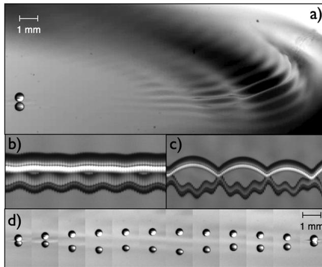
**Figure 12.** (a) Still image of a droplet of 0.5 mm diameter bouncing on a surface oscillating at 188 Hz, the frequency of the rim. Both droplet and bath are 10 cSt silicone oil. Spatio-temporal diagrams indicate the vertical trajectory of droplets of diameter (b) 0.5 mm and (c) 0.35 mm. Time elapses from left to right and the drop's reflection are apparent. (d) A single bounce of a droplet of diameter 0.35 mm is illustrated by an image sequence. Images are spaced by 1 ms.
