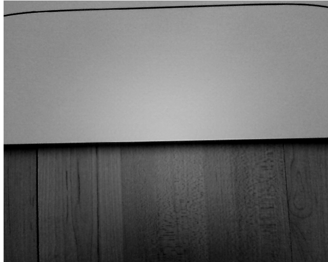
Figure 3.8: Image featuring most curved line, rectified by the parametric algorithm, but still not straight; setup #5
