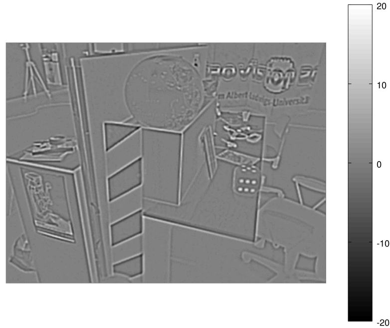
Fig. 2.4. Difference of Gaussians applied to an image from the TUM dataset [45]. Near-zero values indicate feasible edge candidates
