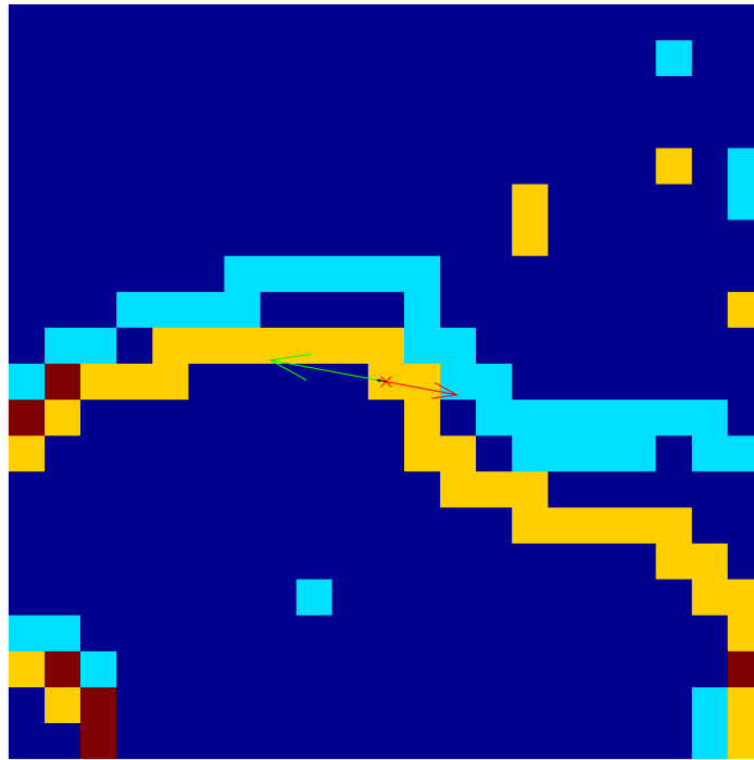
Fig. 2.19. Directed matching along halfline segment. Orange pixels denote current Keylines, rotated to previous frame by \mathbf{R}^T ; cyan – previous Keylines; dark red – position of a current and a previous Keyline. Green and red arrows span over the line segment
