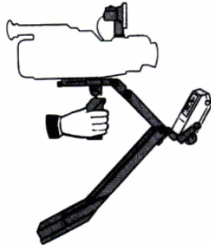
(d) Steadicam Jr. – a compact balanced support, the hand-held version of a Steadicam.
