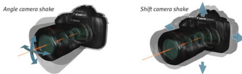
**FIGURE 1.8.** Types of camera shakes.\*
