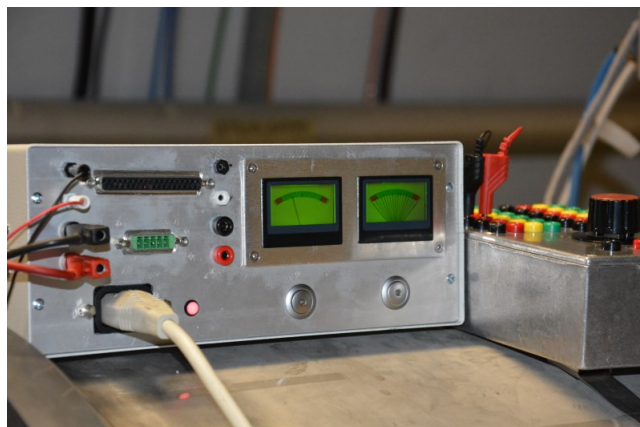
Figure 2.8: Test on machine side, on right side adapter connected to LHC magnet
