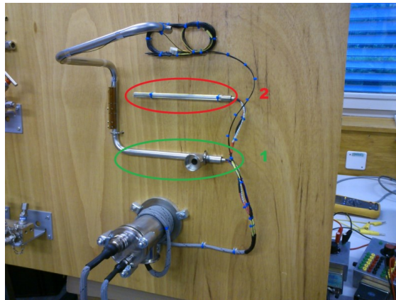
Figure 2.2: Model of heater cartridges, heater and thermocouple sensor inside metal radiator (top) and beam screen cooling line (bottom)
